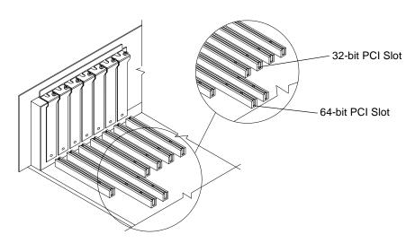
Figure 1-3. 32-bit and 64-bit Expansion Slots
